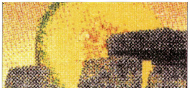
Top to bottom: A printout from the Phaser 440 dye-sublimation printer at 300dpi 24-bit colour (reviewed on page 53), the same image printed on an Epson Stylus Color ink-jet at 720dpi using Acorn's error-diffused printer driver and finally the image printed on the 300dpi Canon BJC-600 ink-jet with a CC TurboDriver which uses simple dithering to mix the colours. All three have been magnified up roughly four times.
